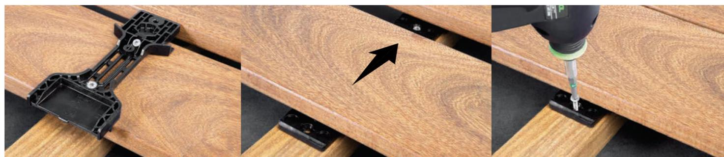
**LES FIXATIONS SONT VISSÉES SUR LE DESSOUS DES LAMES. ELLES SONT ENSUITES VISSÉES "CLASSIQUEMENT" DANS LA LAMBOURDE D'UN SEUL CÔTÉ DE LA FIXATION. L'AUTRE CÔTÉ EST MAINTENU PAR UN SYSTÈME ASSIMILABLE AU FONCTIONNEMENT PAR "RAINURE ET LANGUETTE" AVEC LA FIXATION ADJACENTE.**
